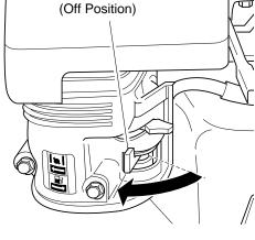
Figure 21 - Fuel Valve Lever Off (Model PGH7500IE Shown)
